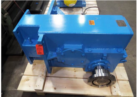
Custom straightener gearbox for steel mill
