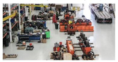
facility with a full in-house machine shop that can handle everything from machining new shafts and spacers to remachining bores in a gearbox housing and can cut spur, helical, double-helical and worm gears.
